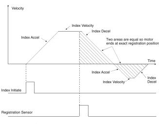
*Figure 46: Registration to Sensor Profile (Offset = 0)*
